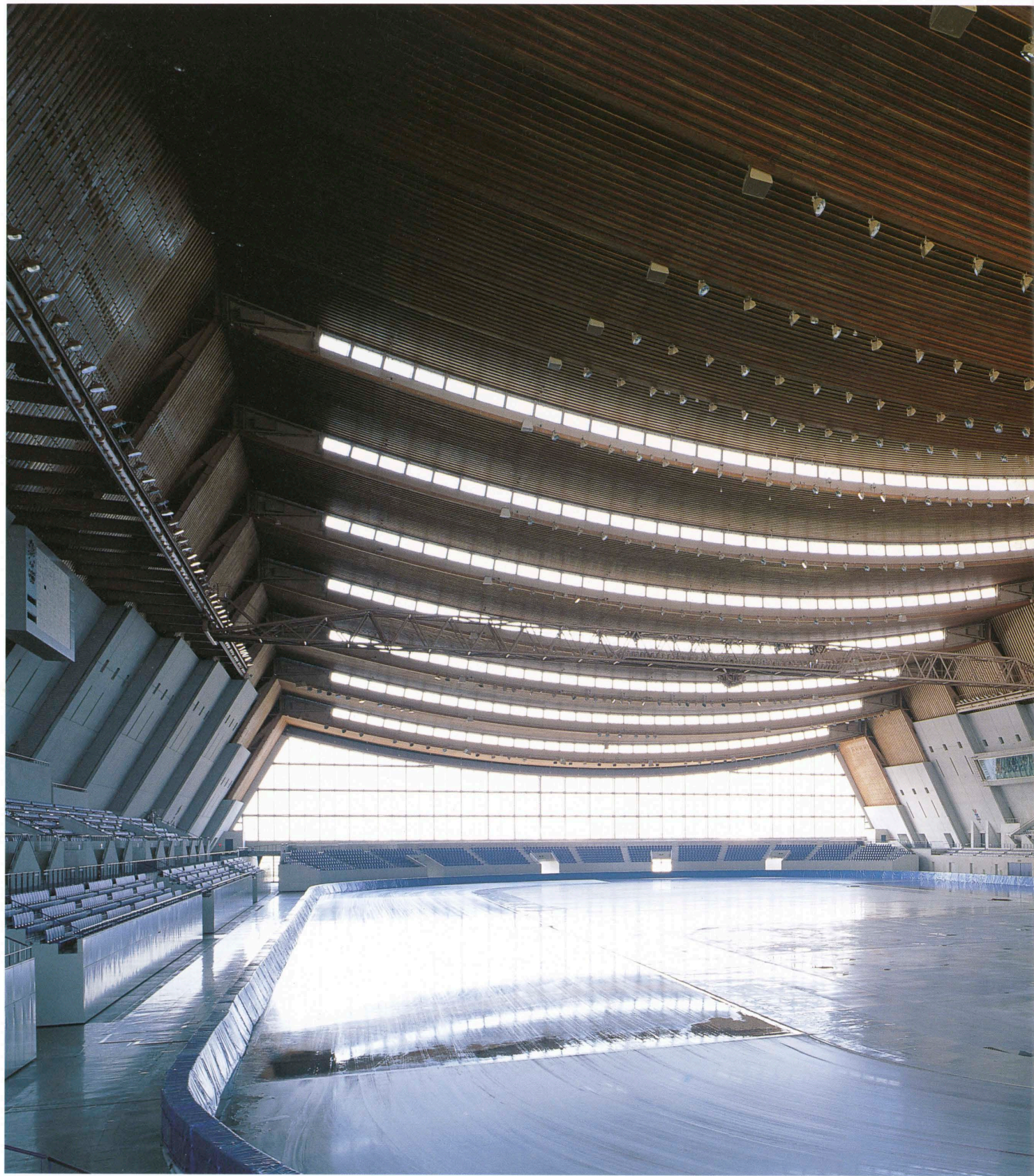
アリーナ内部 信州カラマツ集成材と鋼板による半剛性吊屋根 Interior of the arena. Suspended roof made up of laminated Japanese larch members and steel plates.
